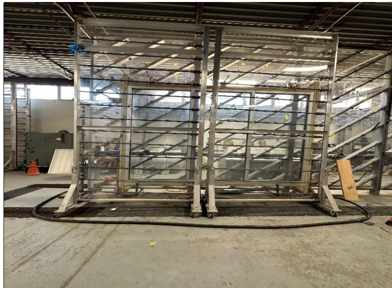
Photo No. 2 Water Penetration Test
